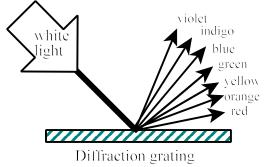
Most spectroscopy instruments use diffraction gratings, instead of prisms, as less light is lost by absorption of the material and the angle of the etched grooves can be precisely controlled. Gratings require less space inside the instrument and can transmit UV radiation. Overall, this results in more speed and resolution per dollar compared to prisms and often a single grating can replace several prisms due to the greater dispersion of radiation.
