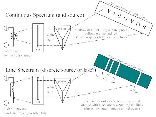
Lasers emit monochromatic light, so no wavelength selector is needed. Discrete and continuous energy sources need additional hardware to isolate the wavelengths of interest.
