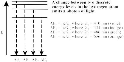
Determining the atomic emission spectrum for each element allows for qualitative identification as each element will have a unique *line spectrum* consisting of a series of separate lines.
