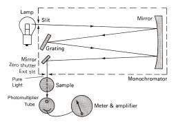
Modern UV-Vis instruments have a tungsten lamp as the white light *source* for the visible region and a deuterium lamp for the ultraviolet region.
