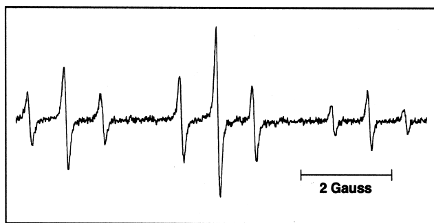
Fig. 5. ESR semiquinone spectrum showing the unique 9-line profile obtained from a crude aspen leaf extract. An indistinguishable spectrum is obtained from a sample of pure catechol, and from pure salicortin, as described in Results. Bar = 2 G.
