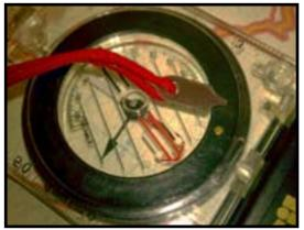
Figure 3: Setting the declination on a typical compass.
