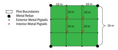
Figure 7: Placing the centre pigtails.
