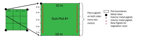
Figure 8: Setting up the subplot grid to sample functional group cover.
