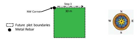
Figure 4: Creating the first corner and measuring one side of the plot (Steps 2-3).
