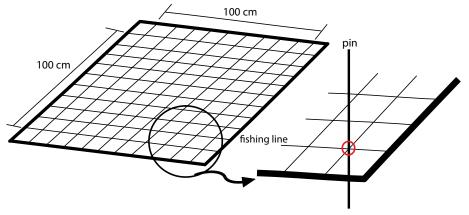
Figure 17: Point frame with inset showing position of pin at the intersection of two strings.
