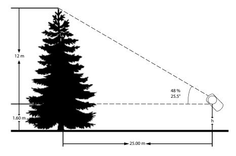
**Figure 13:** Example of how to use a clinometer to determine tree height, where *h* is the height to eye level of the person using the clinometer.
