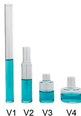
Fig. 1 The four reaction flasks. Nominal interfacial surface areas: V_1 = 1.3 \text{ cm}^2 , V_2 = 2.8 \text{ cm}^2 , V_3 = 5.3 \text{ cm}^2 and V_4 = 10.8 \text{ cm}^2 .
