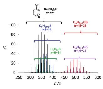
**Fig. 3** ESI mass spectrum of sample B after reaction with **1** in the presence of NaOH. Five distinct product series were observed, which have been colour-coded and labelled with the empirical formula of the reacting species.
