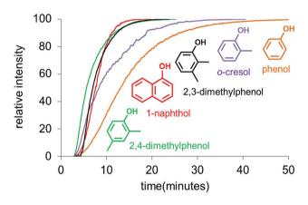
**Fig. 2** Increase in *O*-alkylation products over time, monitored in real time by pressurized sample infusion ESI-MS.
