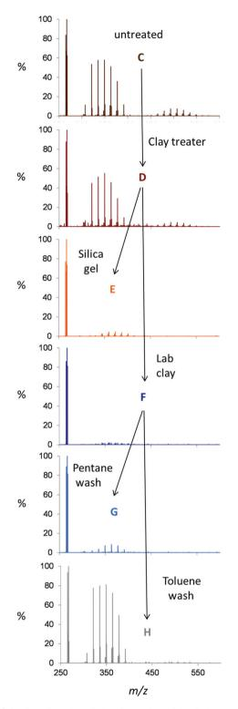
**Fig. 4** Selective phenol analysis of a series of jet fuel samples. The untreated sample (C) is treated with clay, after which spectrum (D) is provided (reduced phenol content). Further treatment with either silica gel (E) or lab clay (F) resulted in much lower phenol content. Washing the lab clay with pentane recovered little phenol (G), but a toluene wash recovered most of it.
