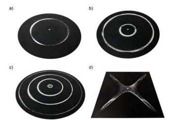
**Figure 3.** Exemplary standing waves produced on Chladni plates. a) 109 Hz, 300 mVpp (2s orbital), b) 354 Hz, 200 mVpp (3s), c) 1690 Hz, 100 mVpp (5s), d) 84 Hz, 100 mVpp  $(3d_{xy})$ .
