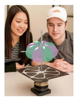
**Figure 2.** A Chladni figure and the corresponding visualized orbital (6g<sub>2</sub>4).
