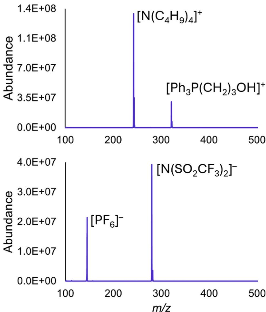
Fig. 2. Positive ion (top) and negative ion (bottom) ESI mass spectra of a 5:5  $\mu\text{mol}$  mixture of  $[\text{N}(\text{C}_4\text{H}_9)_4]^+ [\text{PF}_6]^-$  and  $[\text{Ph}_3\text{P}(\text{CH}_2)_3\text{OH}]^+ [\text{N}(\text{SO}_2\text{CF}_3)_2]^-$  in dichloromethane.
