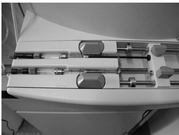
Fig. 8. Photograph showing the double injection system on the ThermoFinnigan LCQ™ DecaXP Plus quadrupole ion trap mass spectrometer which allows co-dilution of samples directly before the sample enters the instrument for analysis.
