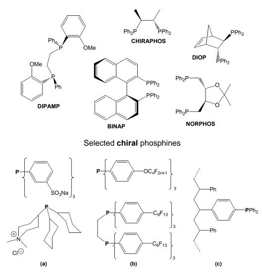
(a) hydrophilic, (b) fluorophasic and (c) polymer-supported phosphines
