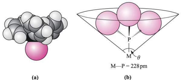
(a) space filling diagram of an M-PPh<sub>3</sub> unit; the phenyl groups adopt a "paddle-wheel" arrangement;
