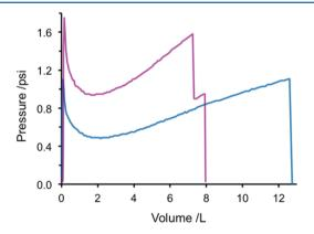
Figure 1. Dependence of balloon pressure on volume of air added during inflation for a single balloon (blue) and double balloon (purple).
