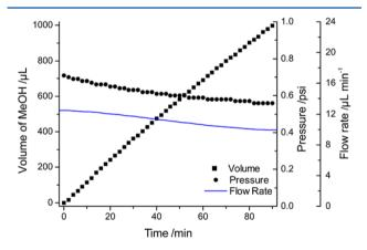
**Figure 2.** Volume of methanol delivered from a double-balloon pressurized Schlenk tube using 178  $\mu$ m ID PEEK tubing over time. Balloon pressure was also monitored. Differentiation of a polynomial best-fit line for the volume data was used to obtain flow rate.
