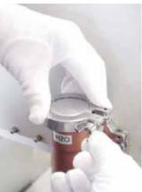
Separate the protective cover on the probe by turning in a counter clockwise direction.
