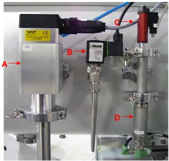
Figure 4 - Antechamber Valve, Gauge & Sensor Assembly
