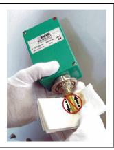
Place an absorbent lint free cloth under the probe and moisten the probe with Phosphoric Acid.
