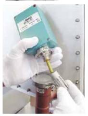
Place an absorbent lint free cloth under the probe and moisten the probe with distilled water.
