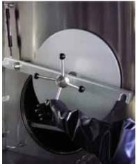
Gently pull out the tray and transfer the material into the glovebox.
