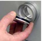
Place the o-ring on the female connector side of the feedthrough.
