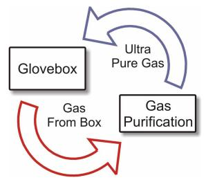
Figure 2 - Principle of Circulation
