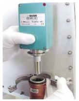
Place a blank KF40 cap over the pipe and secure in place with the clamp.
