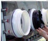
Secure the glove with two o-rings.
