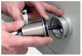
Place the clamp around the flange and tighten.
