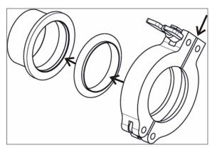
Figure 1 - Clamp, Flange, O-Ring Assembly
