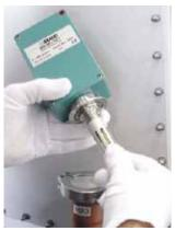
Remove KF40 clamp and blank cap.
