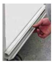
Run the freezer connection cable (G) along the inside of the wire track.
