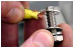
Place the washers onto the bolt with the toothed washer teeth pointing towards the leg of the stand.
