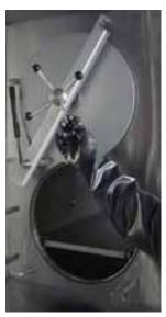
Grasp the door handle with two fingers and turn in a clockwise motion. Tighten finger tight and then an additional ½ turn.
