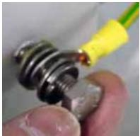
Screw the bolt back into the leg by turning in a clockwise motion.
