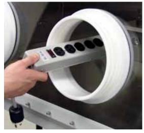
Plug the power strip into the feedthrough.
