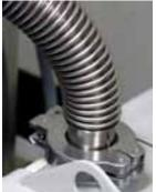
Attach the fitting on the purifier vacuum hose (H) to the port on the copper or stainless pipe and tighten hand tight.
