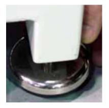
Using a 13mm wrench continue to lower the leveling feet until the casters are raised off the ground.
