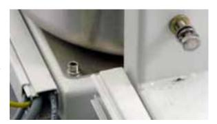
Remove the two bottom washers from the bolt.
