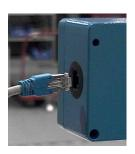
The green plug cable should be wrapped along the circulation pipe and then plugged into the moisture analyzer.
