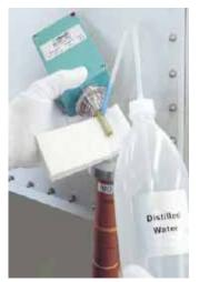
Wrap the moistened cloth around the probe. Gently and slowly spin the cloth around the probe to clean it.
