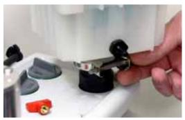
Turn the filter so the label faces the gas ballast on the top of the vacuum pump.
