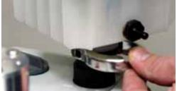
Turn the clamp so the open ends face out.
