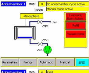
Touch the **Refill** button to refill the antechamber with box gas.
