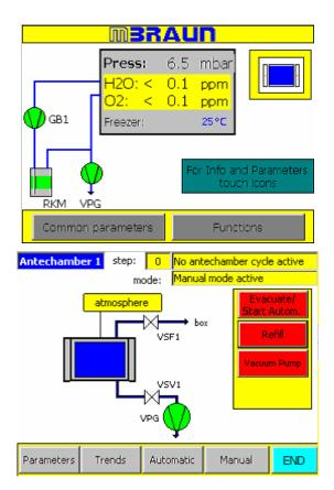
Touch the **Evacuate/Start Autom**. button to evacuate the antechamber of room atmosphere.
