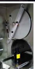
After all materials are transferred into the glovebox, grasp the door handle and gently pull the door down until it rests on the door stop.
