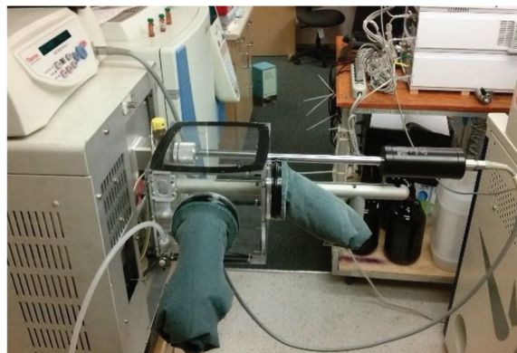
Fig. 1 Left: Schematic of the glove chamber. Right: Glove chamber in place on direct probe EI-MS.
