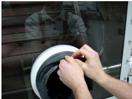
To remove the gloves remove the O-rings and removes the glove as shown
