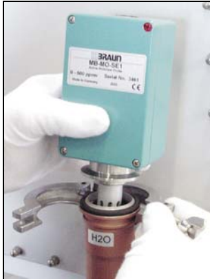
Insert measuring probe and re-clamp.
