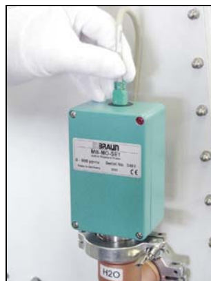
Insert plug connector.
