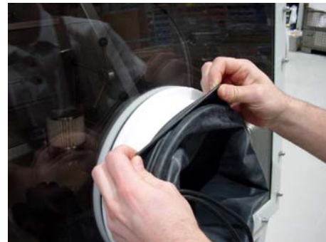
To remove the gloves remove the O-rings and removes the glove as shown
