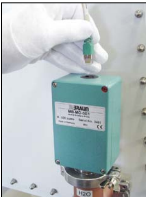
Figure 3: Procedure for Cleaning Moisture Sensor
