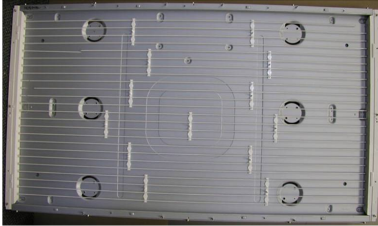
Figure 1.1: Photo of CCFL backlight in conventional LCD display. The light from the fluorescent tubes shines through a diffuser panel which evens it out across the display area. The uniform light then shines through the LCD panel which colours the light and produces the image. [Image courtesy H. Seetzen]
