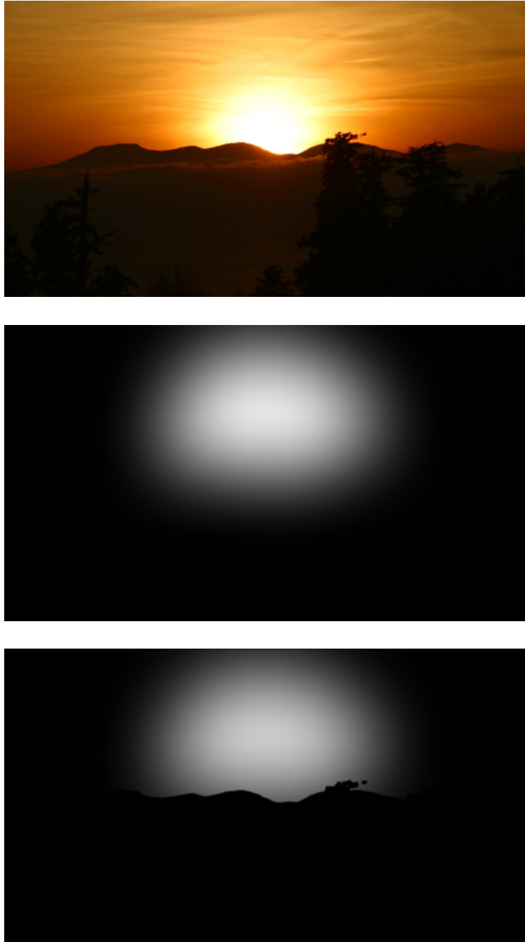
Figure 4.3: Smooth brightness enhancement function (center) and brightness enhancement with edge stopping function (bottom) for an input image (top).
