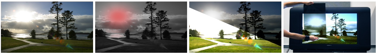
Figure 4.1: Output of our on-the-fly reverse tone mapping algorithm. Left: low dynamic range input image. Center left: a visualization of the brightness enhancement function computed by our method. Center right: two virtual exposures of the resulting HDR image with a contrast of 9300 : 1. Right: the same image shown on an HDR display, using a 10% semi-transparent filter to show details in bright regions.
