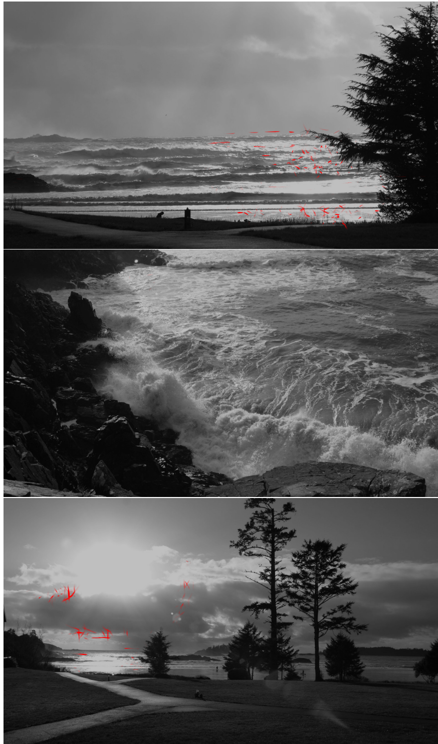
Figure 4.5: Coloured results of the VDP comparison between LDR and HDR image. The red areas show regions that contain pixels that have a 25% probability of being detected as different.
