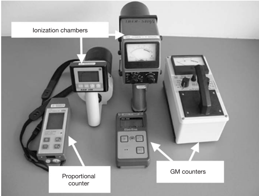
FIG. 4.2. Area survey meters commonly used for radiation protection level measurements: ionization chambers, a proportional counter and GM counters.
