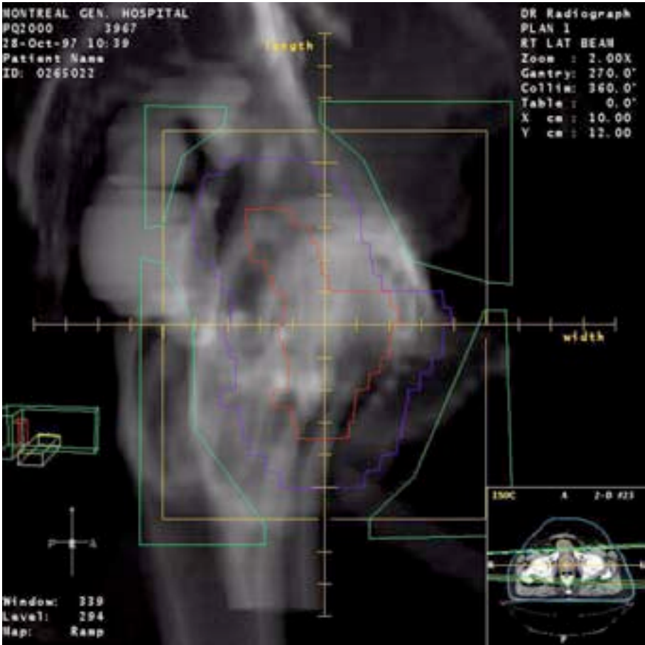
FIG. 7.11. A DRR with superimposed BEV for a lateral field of a prostate patient.
