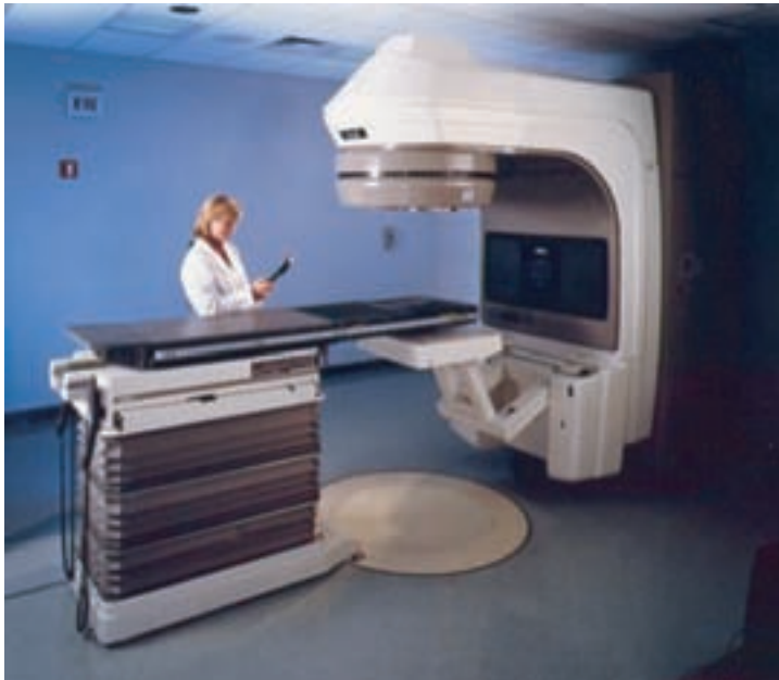
FIG. 5.9. Modern dual photon energy linac manufactured by Varian; the gantry and the patient support assembly are clearly shown. (a) The portal imager is retracted; (b) the portal imager is activated. (Photographs courtesy of Varian Oncology Systems.)
