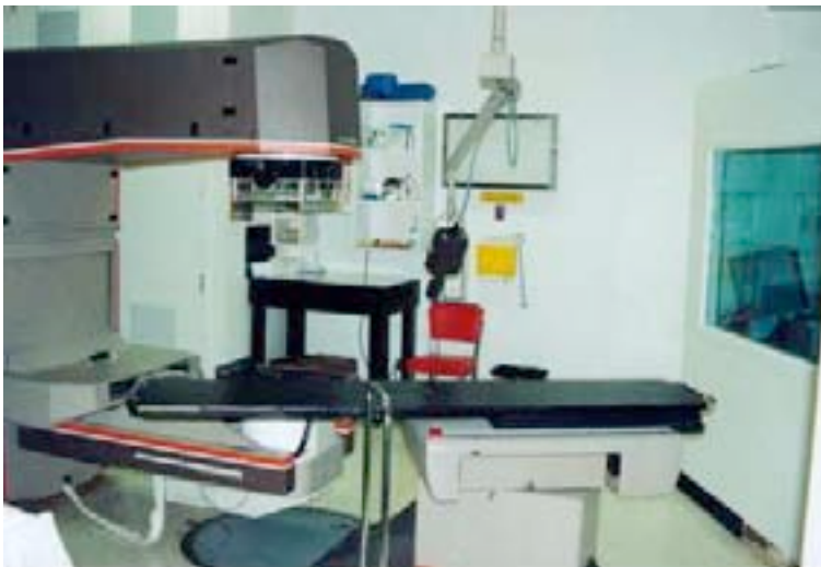
FIG. 7.5. A conventional treatment simulator has the capability to reproduce most treatment geometries available on radiotherapy treatment units. Simulators use a diagnostic X ray tube and fluoroscopic system to image the patient.
