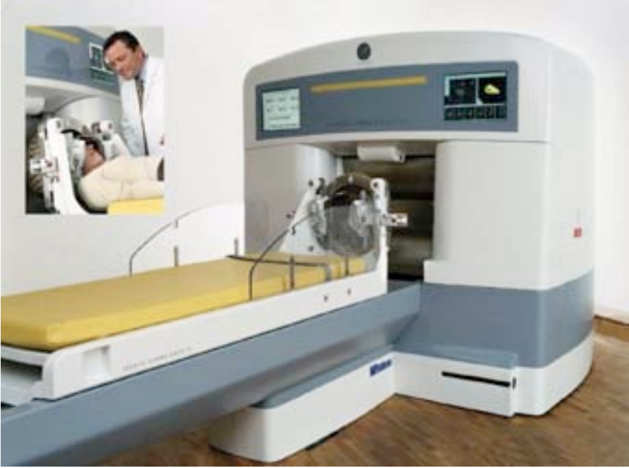
FIG. 15.1. State of the art Gamma Knife (Model 4C) showing the main body of the unit containing 201\text{ }^{60}\text{Co} sources (each nominally with an activity of 30\text{ Ci} = 1.11 \times 10^{12}\text{ Bq} ), the treatment table and a collimator helmet deployed for treatment. The inset shows an up-close image of the automatic positioning system used to position the patient for treatment. (Courtesy of Elekta AB.)
