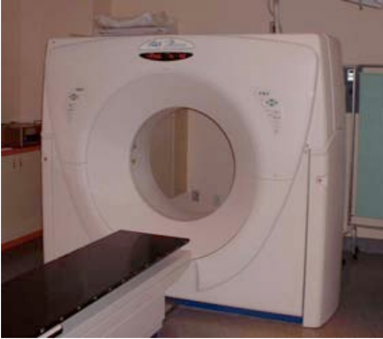
FIG. 7.9. A dedicated radiotherapy CT simulator. Note the flat table top and the large bore (85 cm diameter). The machine was manufactured by Marconi, now Philips.
