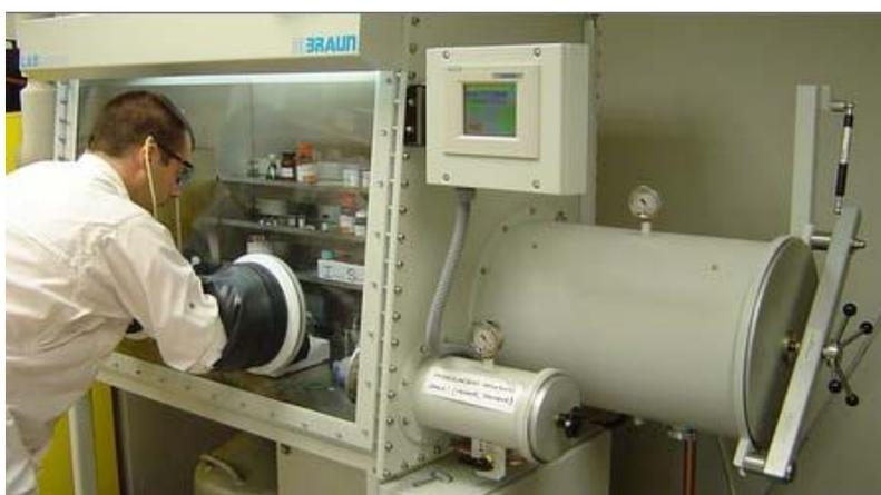
The atmosphere inside the box is continuously purified by passing it through columns containing molecular sieves (removing water) and heated copper metal (removing oxygen).
