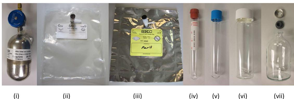
**Figure 1.** Containers tested in this study, including (i) steel canister (Restek, State College, PA, USA), (ii) Tedlar bag (SKC, Eighty Four, PA, USA), (iii) FlexFoil bag (SKC), (iv) Vacutainer (Tyco Healthcare, Mansfield, MA, USA), (v) Exetainer (Labco, Lampeter, UK) with screw-top lid, (vi) EPA vial (Fisher Scientific, Pittsburgh, PA, USA) with screw-top lid, and (vii) glass serum bottle (Wheaton, Millville, NJ, USA) with crimp-top lid.
