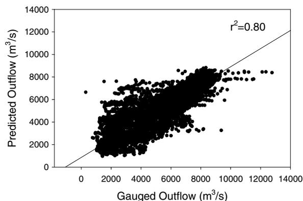
**Figure 3** Measured versus modeled daily outflows from Great Slave Lake for 1964–1998. Modelled outflow is based on the seasonal stage-discharge relationships given in Fig. 2.
