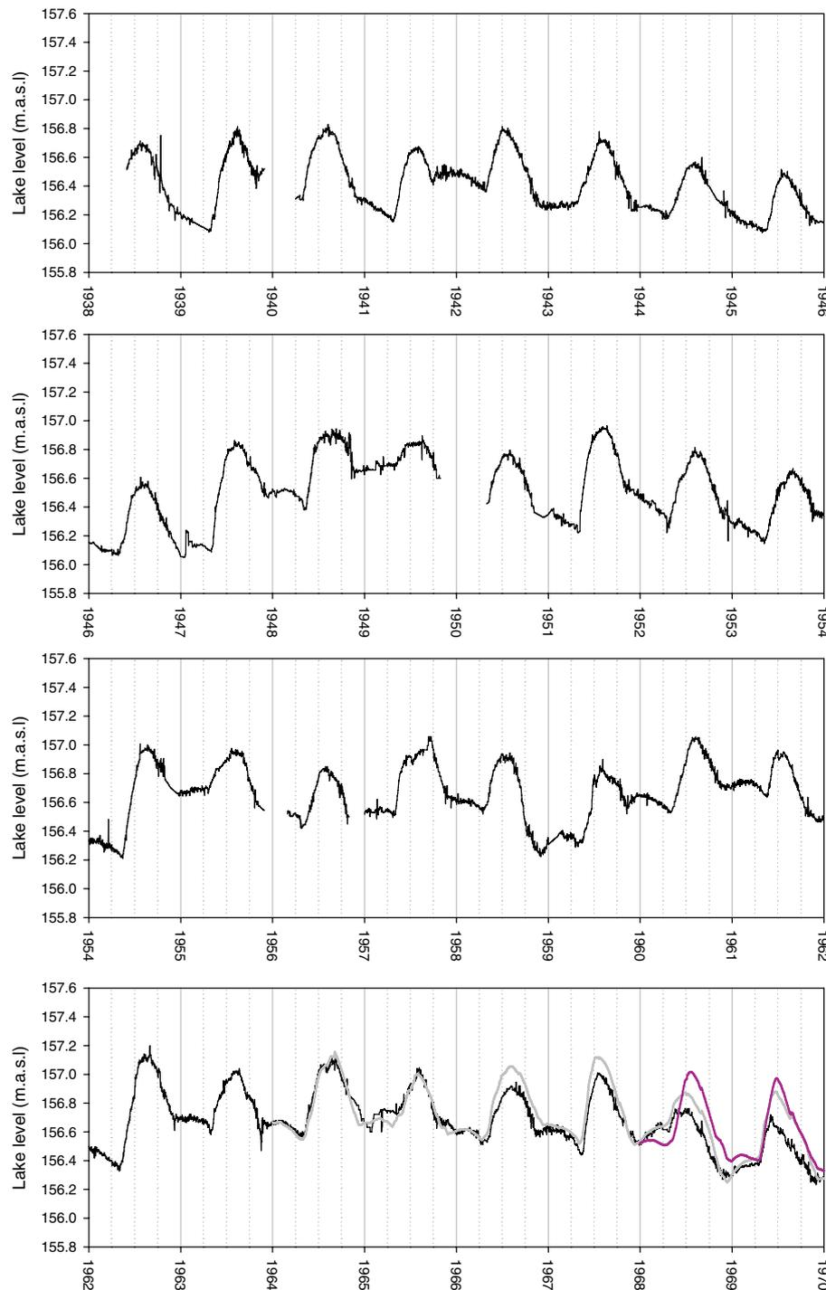
**Figure 4** Observed (heavy black), simulated (grey) and naturalized (thin black) water levels in GSL, 1938–1998.
