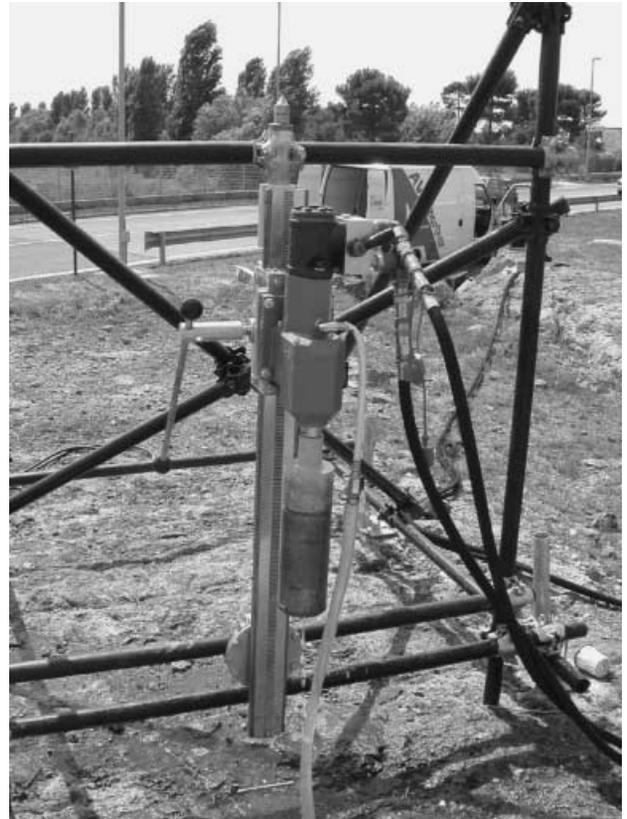
Figure 7. Coring motor and rack, detail.
