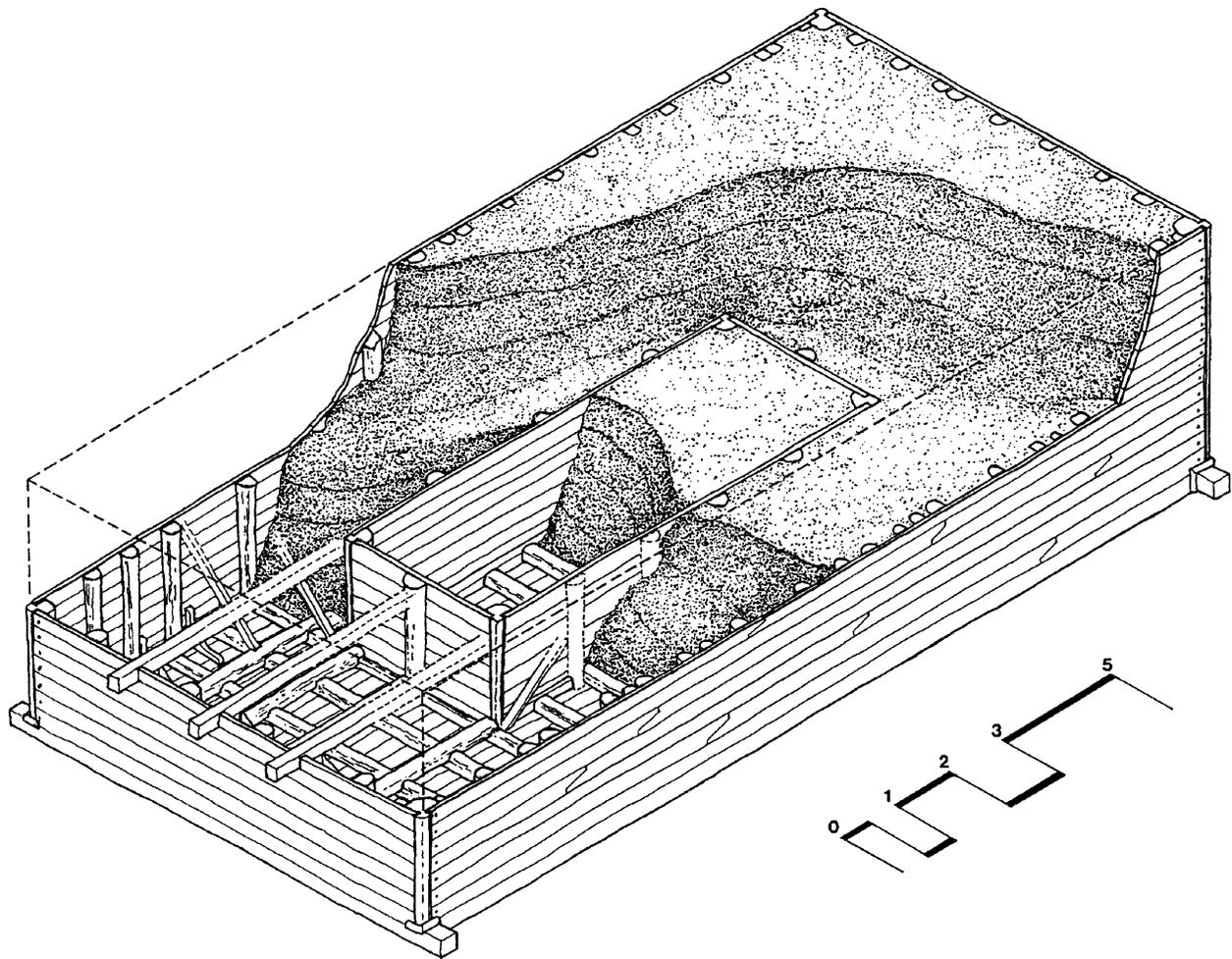
Figure 5. Caesarea: single-use barge formwork. Reconstruction. (C. Brandon)
