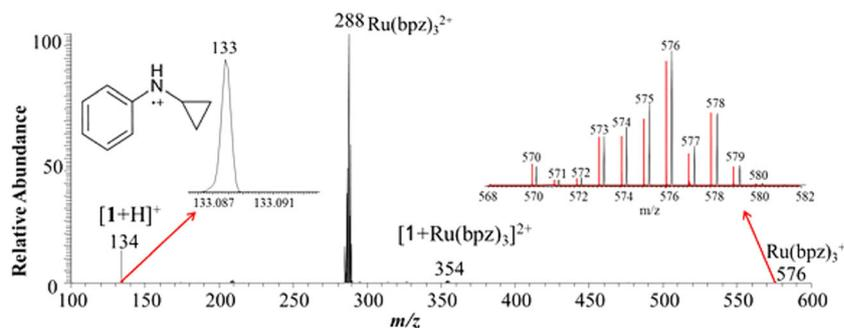
**FIGURE 10** ESI-MS spectrum of Ru(II)  $(\text{bpz})_3(\text{PF}_6)_2$  and N-cyclopropylaniline acquired with light irradiation of the sample. Adapted with permission from study of Cai et al.<sup>24</sup> [Colour figure can be viewed at [wileyonlinelibrary.com](http://wileyonlinelibrary.com)]
