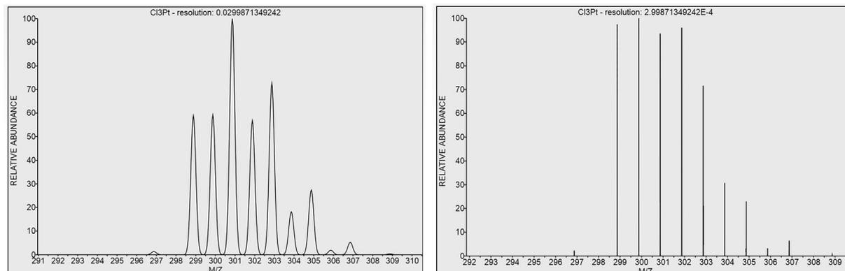
**FIGURE 5** Isotope patterns calculated at different resolutions for  $[\text{PtCl}_3]^-$ : 1000 (left) and 100 000 (right)
