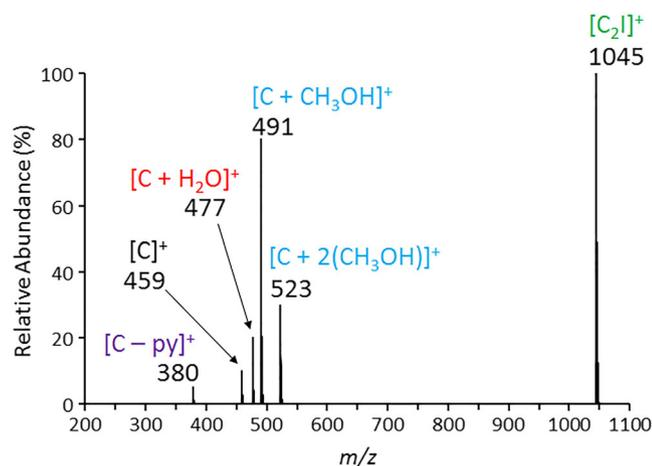
**FIGURE 7** Simulated spectrum showing commonly observed signals for a generic cation,  $C^+$ : The bare ion (459 Da, black), solvated ions (blue), a cluster ion (green), an adventitious adduct (red), and a neutral loss (purple, py = pyridine). Peak intensities are hypothetical and may vary dramatically
