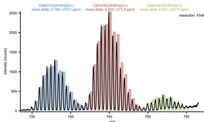
**FIGURE 4** Isotope pattern matching for three related dipalladium dications [Colour figure can be viewed at [wileyonlinelibrary.com](http://wileyonlinelibrary.com)]
