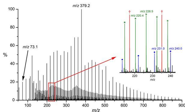
**FIGURE 11** Positive ion electrospray ionization mass spectrum of an aqueous solution of  $\text{LaCl}_3$  before peak assignment. Adapted from the study of McQuinn et al.<sup>34</sup> [Colour figure can be viewed at [wileyonlinelibrary.com](http://wileyonlinelibrary.com)]
