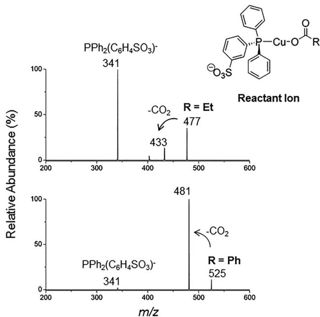
**FIGURE 6** MS/MS spectra of  $[\text{Cu}(\text{PPh}_2(\text{C}_6\text{H}_4\text{SO}_3))(\text{CO}_2\text{R})]^-$  where  $R = \text{Et}$  (top,  $m/z$  477) and  $R = \text{Ph}$  (bottom,  $m/z$  = 525). Adapted from the study of Vikse et al.<sup>17</sup>
