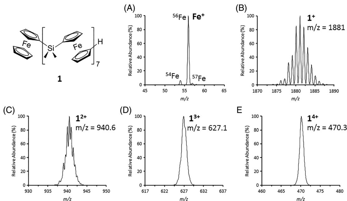
**FIGURE 2** Simulated spectra of  $\text{Fe}^+$  and **1** in various oxidation states
