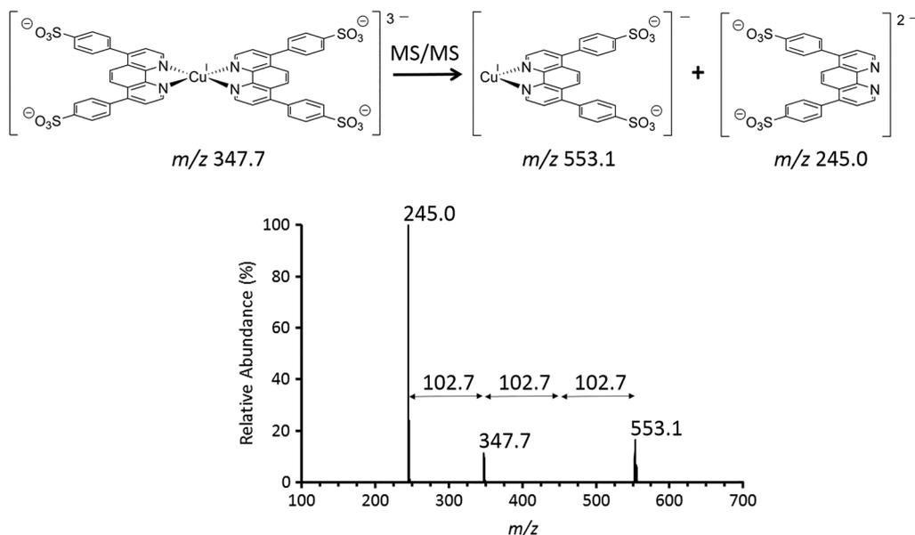
**FIGURE 8** Scheme (top) and MS/MS spectrum (bottom) of the fragmentation of a triply-charged copper complex ( $m/z$  347.7)
