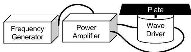
Figure 1. Schematic of the demonstration setup.
