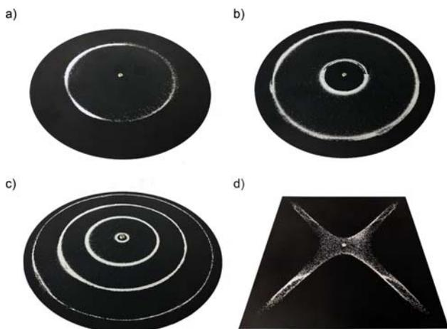
**Figure 3.** Exemplary standing waves produced on Chladni plates. a) 109 Hz, 300 mVpp (2s orbital), b) 354 Hz, 200 mVpp (3s), c) 1690 Hz, 100 mVpp (5s), d) 84 Hz, 100 mVpp (3d<sub>xy</sub>).
