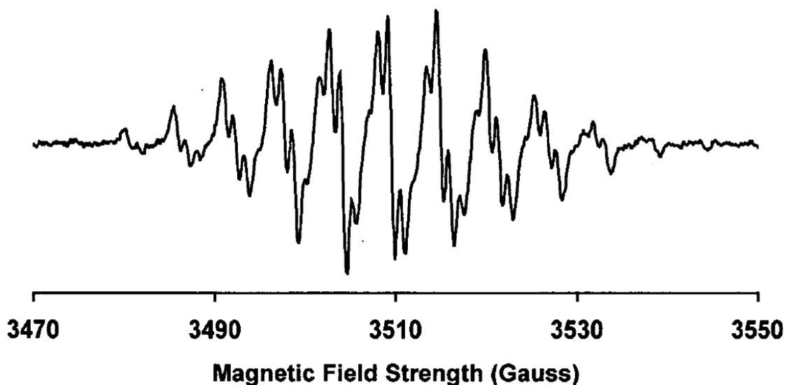
An **electron paramagnetic resonance** (EPR) spectrum. The technique can reveal information about the symmetry of the complex and how the unpaired electron is delocalised.
