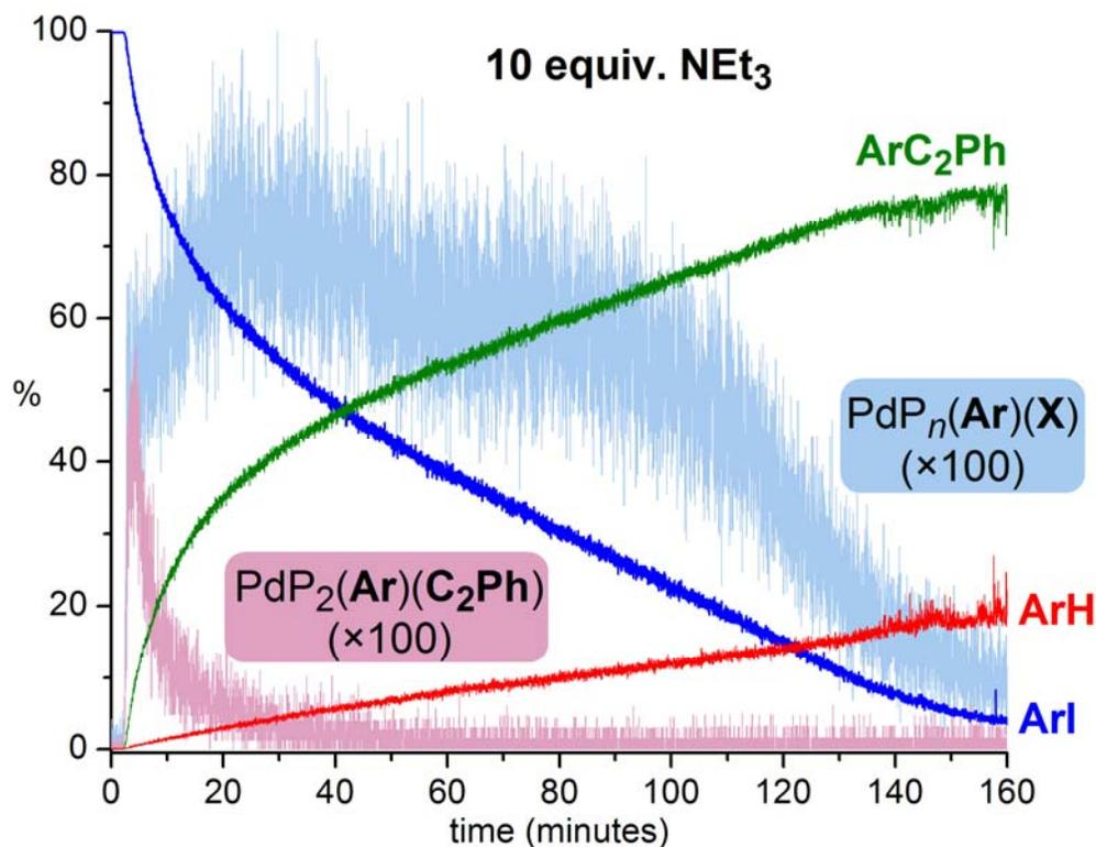
ESI-MS intensity data over time for all key species containing Ar = [*p*-C<sub>6</sub>H<sub>4</sub>CH<sub>2</sub>PPh<sub>3</sub>]<sup>+</sup> [PF<sub>6</sub>]<sup>-</sup> in a copper-free Sonogashira cross-coupling reaction. The intensity of the Pd-containing intermediates (P = PPh<sub>3</sub>) has been multiplied by 100.
