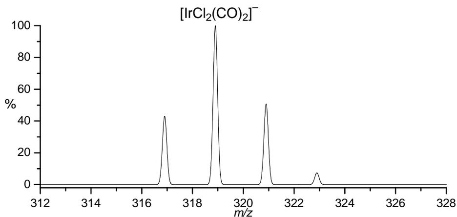
Calculated isotope pattern of  $[\text{IrCl}_2(\text{CO})_2]^-$ .
