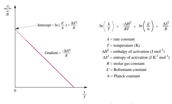
An **Eyring plot** allows the activation parameters  $\Delta S^{\dagger}$  and  $\Delta H^{\dagger}$  to be determined from the temperature dependence of the rate constant; the dotted part of the line represents an extrapolation.
