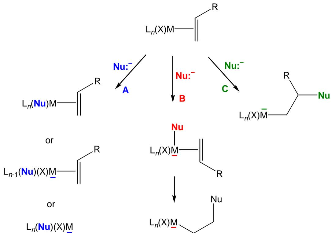
Possible **reactions of nucleophiles**. Path **A**: nucleophilic attack at the metal. **B**: nucleophilic attack at the metal followed by syn insertion of an unsaturated ligand. **C**: nucleophilic attack at the ligand.
