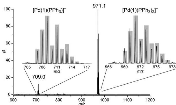
**Fig. 1** Negative-ion ESI-MS of  $Pd(PPh_3)_4 + [PPN][I]$  in  $CH_2Cl_2$ . Insets: isotope pattern matching for  $[Pd(PPh_3)_n]^-$  ( $n = 1$  and  $2$ ).
