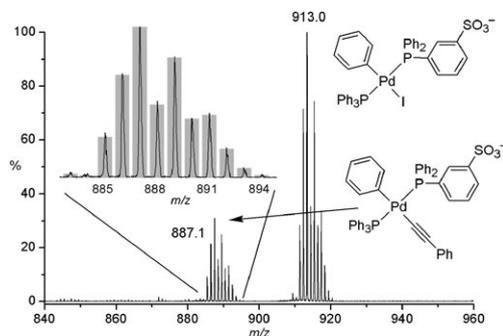
**Fig. 2** Negative-ion ESI-MS of  $Pd(PPh_3)_4 + [PPN][I] + 100 \times (PhI + PhC_2H + NEt_3)$  in  $CH_2Cl_2$ . Inset: isotope pattern match for  $[Pd(II)(PPh_3)(Ph)(C_2Ph)]^-$ .
