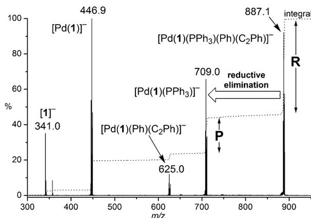
**Fig. 3** Negative-ion ESI-MS/MS of  $[\text{Pd}(\text{I})(\text{PPh}_3)(\text{Ph})(\text{C}_2\text{Ph})]^-$ , showing reductive elimination of  $\text{PhC}_2\text{Ph}$ , at a collision voltage of 15 V.
