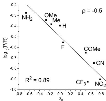
**Fig. 4** Plot of  $\log_{10}(P/R)$  vs. Hammett  $\sigma_p$  parameter.
