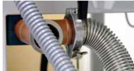
Attach the “Out” KF40 stainless steel flexible hose (C) on the blower to the bottom of the heat exchanger using a KF40 clamp and o-ring.
