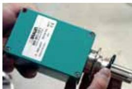
Carefully place the sensor end of the analyzer into the corresponding port on the circulation piping running the length of the system on the underside of the glovebox.
