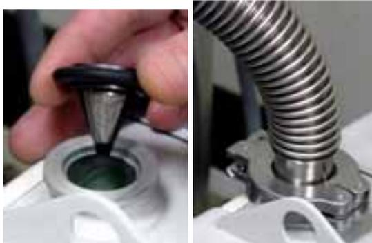
Attach the fitting on the purifier vacuum hose (H) to the port on the copper or stainless pipe and tighten hand tight.
