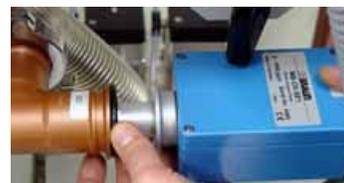
Secure the analyzer to the pipe using a KF-40 clamp and o-ring.
