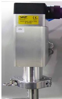
Attach the stainless steel flexible hose to the port on the vacuum pump with the funnel shaped o-ring using a KF25 clamp.
