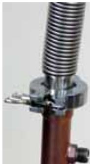
Attach the pipe to the valve located on the bottom of the rear side of the antechamber using a KF40 clamp and o-ring.
