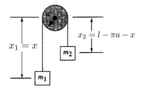
Pulley has moment of inertia I; hence we have two Cartesian coordinates plus the constraint  $x_1 + \pi a + x_2 = l$  (l is the length of the cord).
