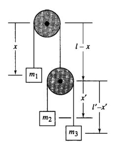
**Example 4**: The Double Atwood Machine (neglect pulley radii)
