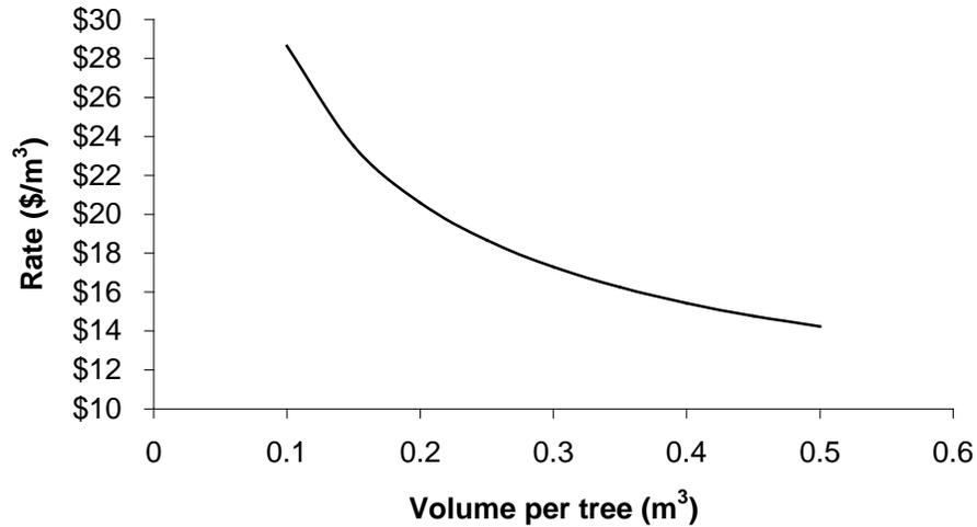
Figure 1: Logging rates ( $\$/\text{m}^3$ ) by volume per tree.
