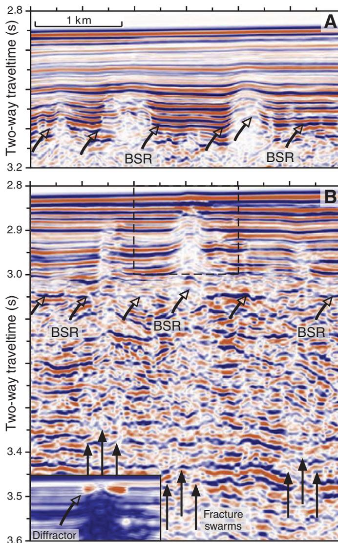
**Figure 2.** Detailed seismic reflection sections from two boxed areas of Figure 1. Inset (B) is envelope amplitude of dashed area. Steep amplitude striations in and beneath vent feature B are fractures referred to in text. BSR—bottom-simulating reflector.
