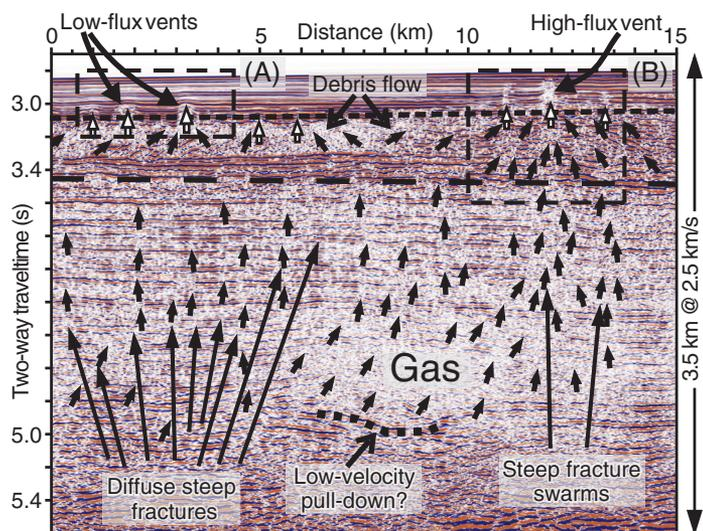
**Figure 1.** Time-migrated section from line KIGAM UBGH-043. Two vent structures discussed in text and shown in Figure 2 are marked here by dashed boxes. Processing flow includes normal moveout (NMO) corrections and stacking, frequency filtering between 20 and 250 Hz, finite-difference time migration, and time-dependent (laterally invariant) exponential gain. Uninterpreted seismic reflection image used to produce this figure is available in the GSA Data Repository.<sup>1</sup>
