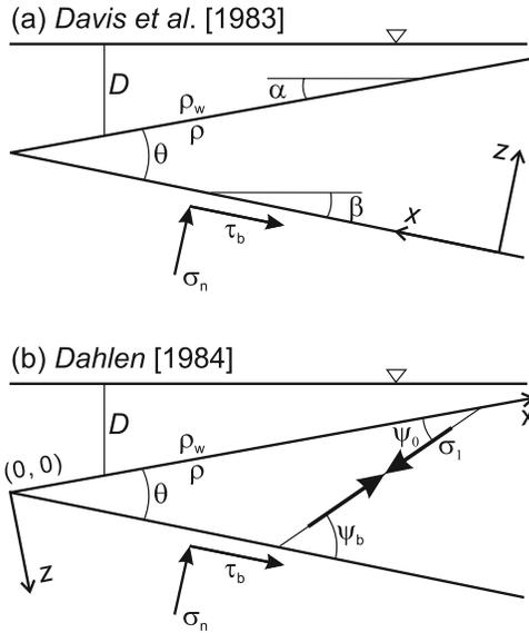
**Figure 1.** Schematic illustration of coordinate systems used in the Coulomb wedge theory ( $x, z$ ), maximum compressive stress  $\sigma_1$ , angles  $\alpha, \beta, \theta, \psi_o$ , and  $\psi_b$ , water depth  $D$ , and basal tractions.  $\rho$  and  $\rho_w$  are densities of the wedge material and overlying water, respectively.
