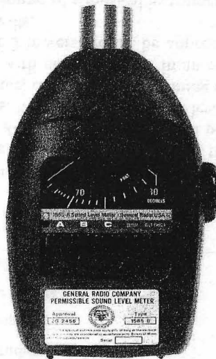
Figure 8-1 The intensity of sound or noise is measured with a sound-level meter ( bottom ). The meter does not ordinarily add the power of all frequency components of the sound and measure the sum. Rather, it “weights” the powers of different frequency components before adding. Weighting curve A ( top ) is commonly used, because the reading so obtained is closely related to loudness to the human ear for sounds of moderate intensity. Sound levels measured using the A setting (and weighting) of a sound-level meter are often quoted as dBA, as, for example, a noise level of 40 dBA. To measure the actual power of a sound, we would use the C weighting. The B weighting lies between A and C and would be appropriate for quite intense sounds.
