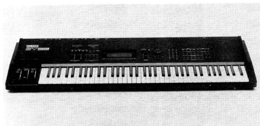
Figure 1-10 The Yamaha SY99, a late model digital keyboard. The earlier Yamaha DX7, which reached the market in 1983, was the first completely digital keyboard synthesizer, and the first such synthesizer that sold at an affordable price (around $2,000). Early “digital” keyboard devices sold for about ten times this price. The success of the DX7 was due partly to Japanese persistence and ingenuity, partly to the use of special integrated circuit chips, and partly to the use of fm (frequency modulation) synthesis, an invention of John Chowning. Now discontinued, the DX7 was a landmark that ushered in a new era. (Photo courtesy of Yamaha Corp. of America)
