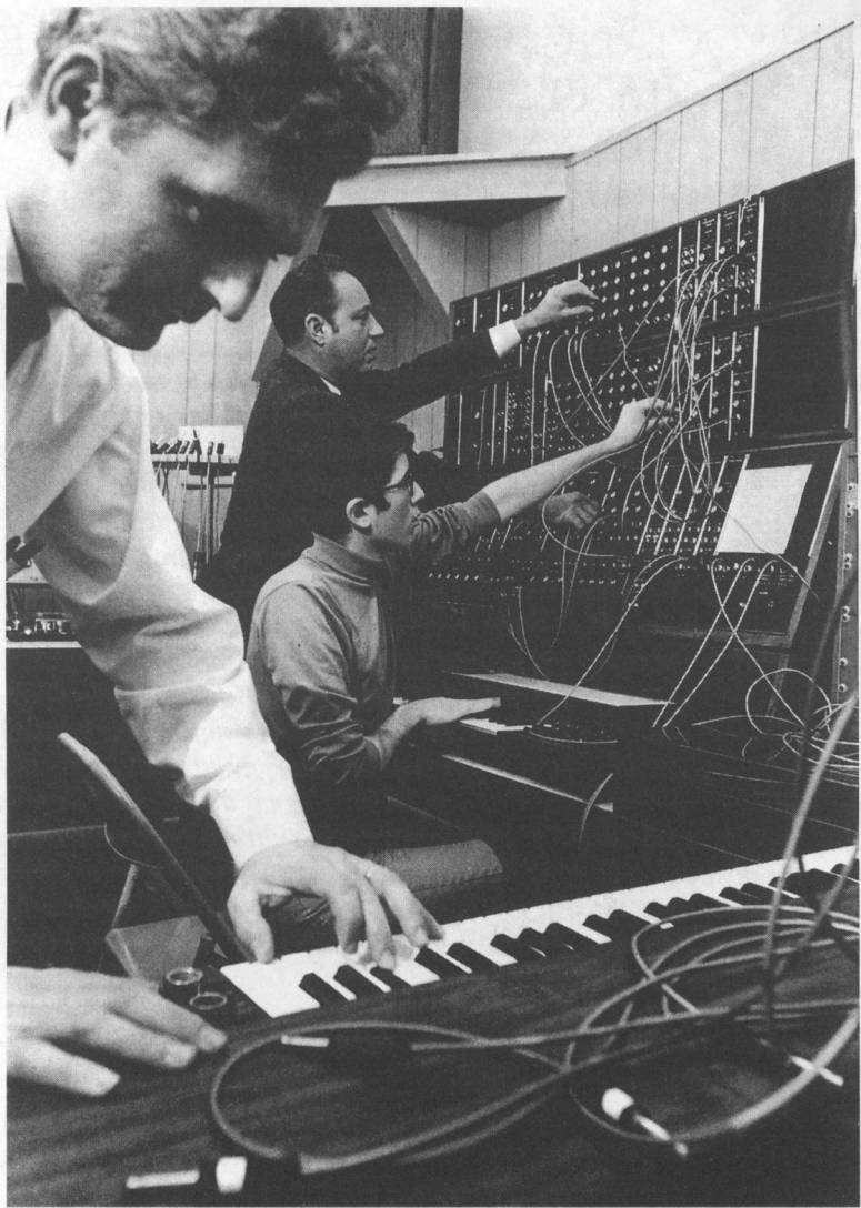
Figure 1: This is an early promotional picture used by the R.A. Moog company showing a Series 900 modular synthesizer. It is being demonstrated by Bob Moog, the individual in the foreground, Frank Harris, at the back, a musician from St. Louis, and Jon Weiss, the young man sitting down, a musician who started with Moog as a work study student. Photograph courtesy of R.A. Moog.
