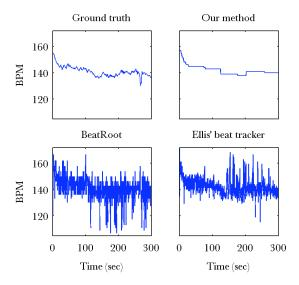
**Figure 2**. Four estimates of the tempo curve for our recording *CB*: Ground truth calculated from a human expert's tap times (upper left), curve from our method (top right), curve from BeatRoot (lower left), and curve from Ellis' dynamic programming approach (lower right).
