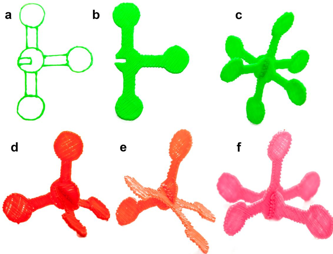
**Figure 2.** Top: the three stages of the octahedral model construction from the template: (a) outline, (b) infill, (c) assembly. Note that after the infill process, the plastic blocking the notch on the central atom of the outline needs to be cut away with scissors before assembly. Bottom: examples of the final product obtained, based on (d) four (tetrahedral), (e) five (trigonal bipyramidal), and (f) six (square pyramidal) electron domains. Photo credit: Kari Matusiak.
