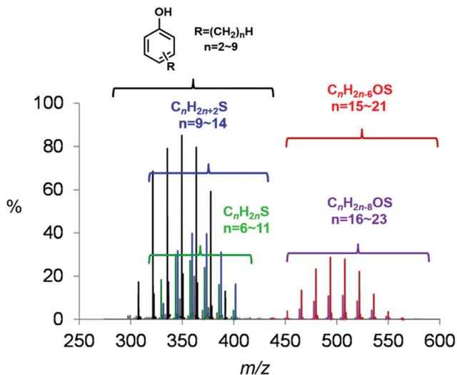
**Fig. 3** ESI mass spectrum of sample B after reaction with **1** in the presence of NaOH. Five distinct product series were observed, which have been colour-coded and labelled with the empirical formula of the reacting species.
