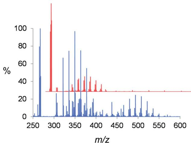
Fig. 5 Jet fuel sample X2 before (blue) and after (red) stirring in the presence of alumina for 40 hours.
