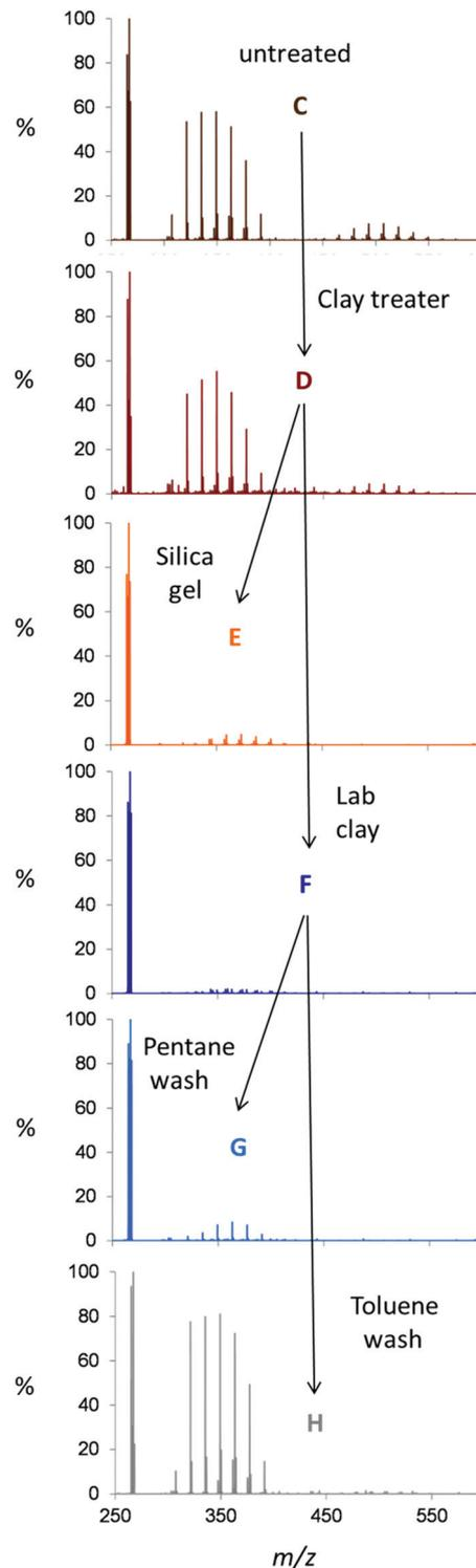
**Fig. 4** Selective phenol analysis of a series of jet fuel samples. The untreated sample (C) is treated with clay, after which spectrum (D) is provided (reduced phenol content). Further treatment with either silica gel (E) or lab clay (F) resulted in much lower phenol content. Washing the lab clay with pentane recovered little phenol (G), but a toluene wash recovered most of it.
