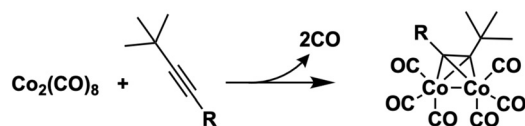
Fig. 1 The formation of CCTBA. This reaction can be performed neat or in a non-polar solvent at room temperature.
