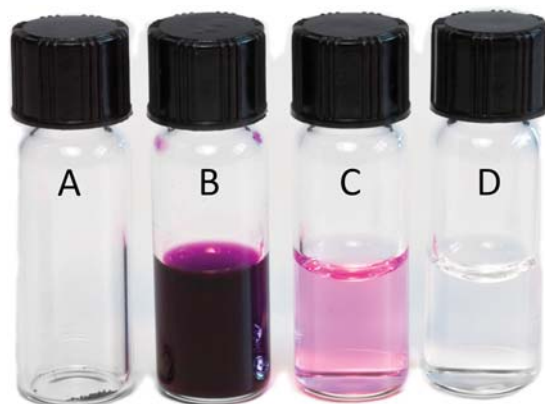
Figure 2. A milligram of sample (A), dissolved in 1 ml of solvent (B), diluted by a factor of 20 (C) and further diluted by a factor of 20 (D).
