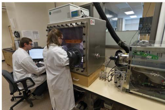
Figure 4. Glovebox adjacent to the ESI-MS. The syringe pump in use is located inside the glovebox.
