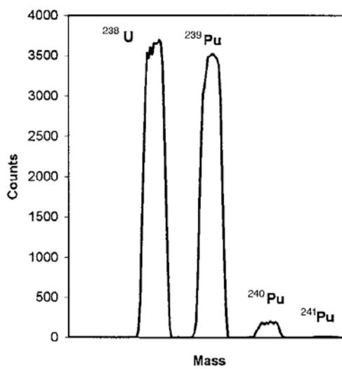
**Figure 8.** ICP-MS trace for a  $10 \text{ pg ml}^{-1}$   $^{239,240}\text{Pu}$  standard solution with a  $^{240}\text{Pu}/^{239}\text{Pu}$  ratio of 0.054.
