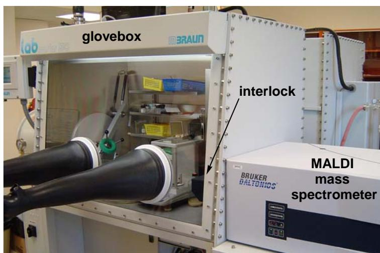
**Figure 9.** Mass spectrometer interfaced with an inert-atmosphere glovebox. Photo taken in the laboratory of Prof. D. Fogg, University of Ottawa.
