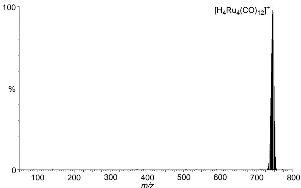
**Figure 3.** LIFDI spectrum of  $\text{H}_4\text{Ru}_4(\text{CO})_{12}$ . Spectrum provided by H. B. Linden.
