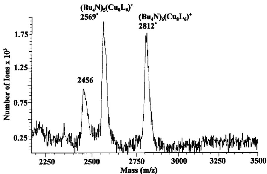
**Figure 4.** The positive ion  $^{252}\text{Cf}$ -PD mass spectrum of  $[\textit{n}\text{-Bu}_4\text{N}]_4[\text{Cu}_8(\text{S}_2\text{CC}(\text{CN})_2)]$  adsorbed on Hybond N+. Adapted with permission from reference 8.
