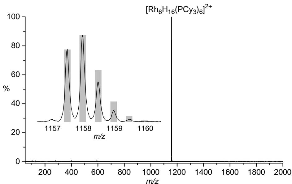
**Figure 6.** Positive-ion ESI-MS of  $[\text{Rh}_6\text{H}_{16}(\text{PCy}_3)_6]^{2+}$  in dichloromethane. The inset shows calculated and experimental isotope patterns. Note the lack of fragmentation. Used with permission from reference 17.
