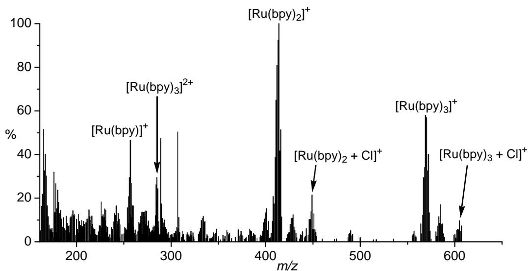
**Figure 5.** Positive-ion LSIMS of [Ru(bipyridine)<sub>3</sub>]Cl<sub>2</sub> in a 3-nitrobenzyl alcohol matrix. Adapted with permission from reference 1.
