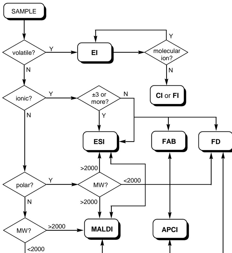
**Figure 10.** Flowchart for choosing an ionization technique based on the properties of the sample. LSIMS is treated as synonymous with FAB. PDMS is rare so does not appear; it can handle similar types of samples as does MALDI. ICP-MS can handle all sample types, but provides no molecular weight information and so is not included.
