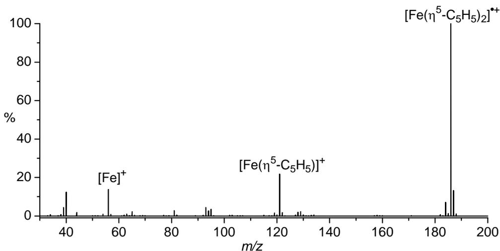
**Figure 1.** EI mass spectrum of ferrocene. Unusually, the molecular ion is the base peak. Adapted with permission from reference 1.
