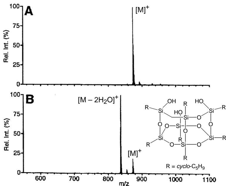
**Figure 2.** APCI-MS for (a) heptacyclopentyl- $T_7$ -silsequioxane ( $m/z$  875) and (b) CID spectrum yielding a base peak at  $m/z$  857 corresponding to loss of  $2H_2O$ . Adapted from reference 4 with permission.
